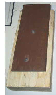
c) Shear failure of fixing in Timberstrand LSL flitch connection
