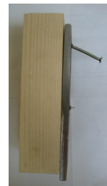
a) Bending failure of fixing in C24 flitch connection
