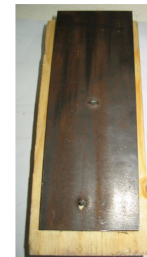
b) Shear failure of fixing in LVL flitch connection
