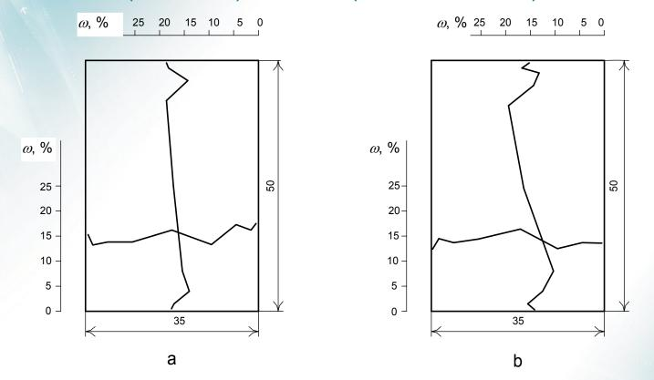
Significant moisture content variations occur in timber surface layers. Similar proportion could be expected for shrinkage stresses values in these layers.
