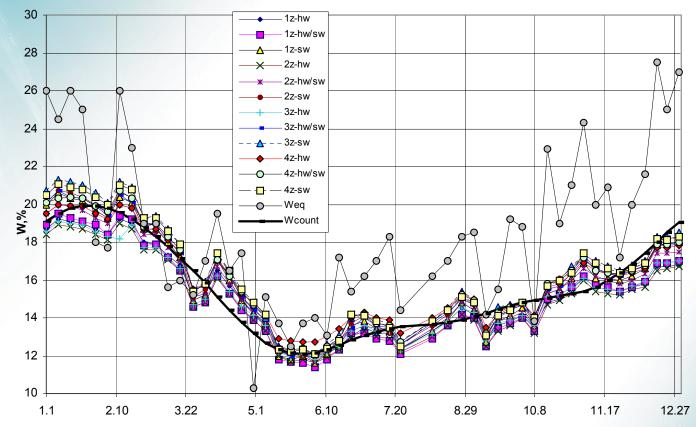
Test samples were cut from central yield boards at four different height zones - *1z, 2z, 3z,* and *4z* - of the tree stem (1 zone - near the stump, 2 zone - 3,2-3,7 m, 3 zone - 6,3-6,8 m, 4 zone - 9,5-10 m away from the stump), while transversely - from heartwood (*hw*), from sapwood (*sw*) and partly from heartwood - partly from sapwood (*hw*-*sw*).
