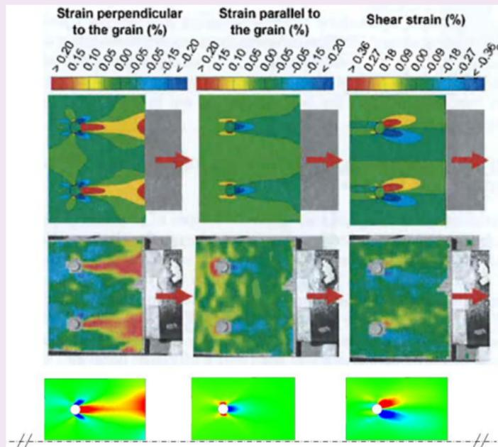
**F=3.5 kN (25% of the experimental elastic limit). Load applied for 1 month. Cases of drying and wetting.**
