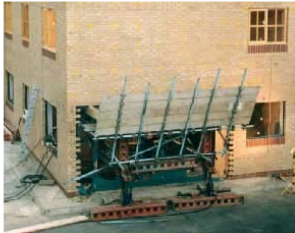
Figure 5. Test of timber frame
