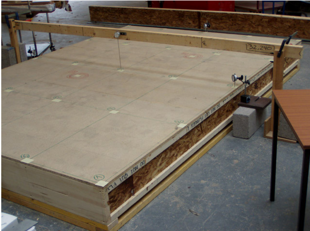
Figure 2: Typical British floor built with I-joists and chipboard deck for a deflection test
