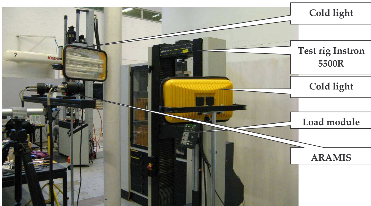
Figure 6: Experimental set-up with ARAMIS
