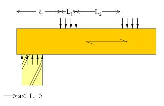
Tension perpendicular to the grain (and shear?)
