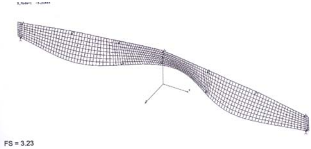
Figure 20 Bucking of girder
