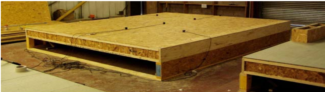
Figure 3 — Setup for a measurement of the dynamic floor response
