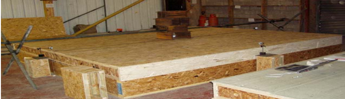
Figure 2 — Setup for a deflection test
