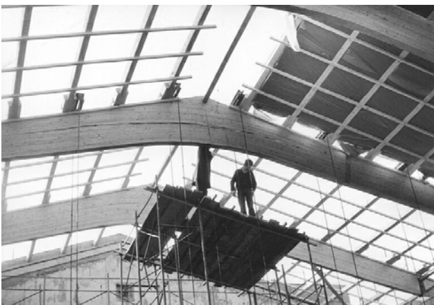
Figures 5, 6: Failure of beam during in-situ loading test
