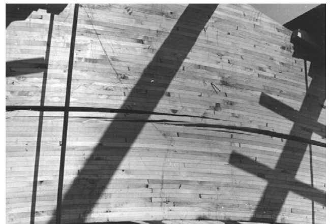
Figures 5, 6: Failure of beam during in-situ loading test
