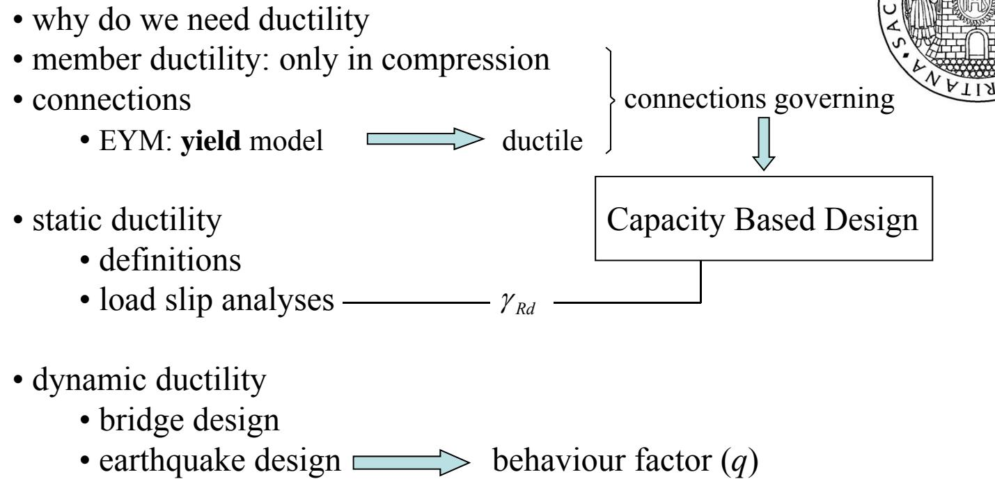
$$\text{design seismic action} = \frac{\text{real seismic action}}{q}$$
